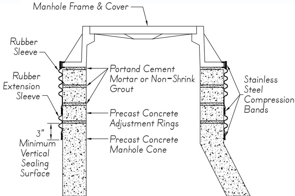
**PRECAST MANHOLE WITH EXTERNAL SEAL**
